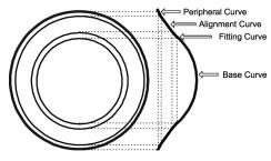
Figure 1: Representation of the reverse geometry lens design
